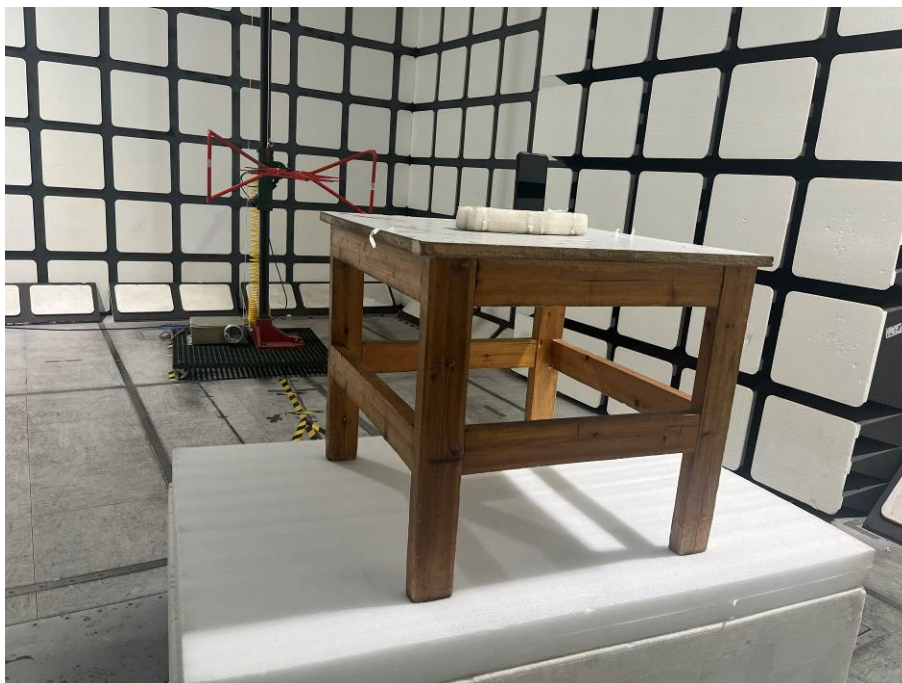
Radiated Spurious Emissions Test View (Above 1GHz)
