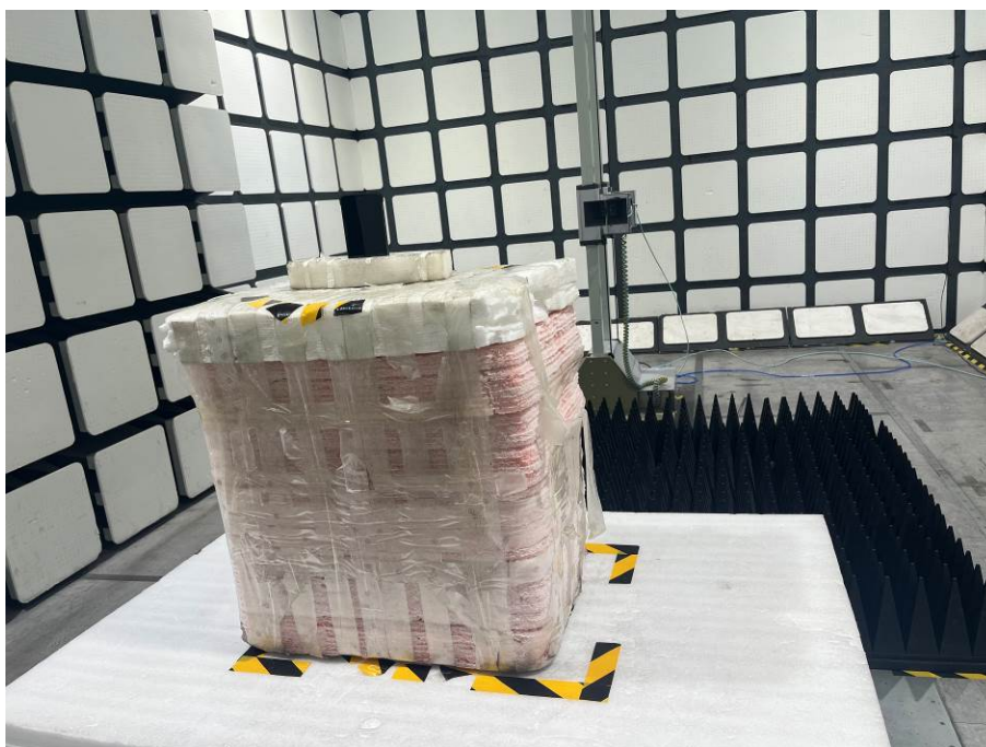
Radiated Spurious Emissions Test View (Above 1GHz)
